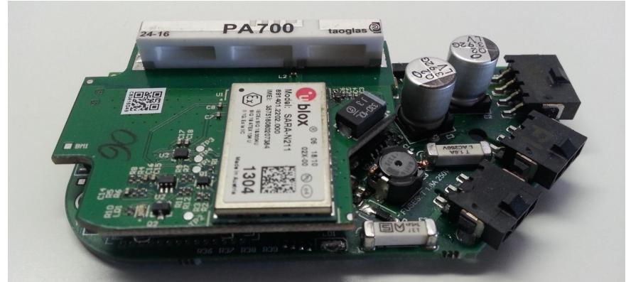
3phase **smart meter** with WiFi, GSM / UMTS / NB-IoT connectivity: hardware design, certification approval (EN61010, EMC, RED)
