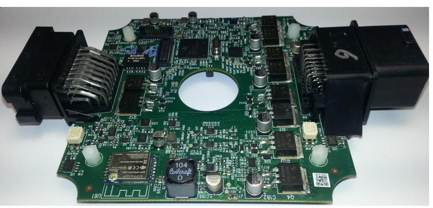
8 layers **proportional valves driver** with WiFi, CAN, ethernet connectivity for automotive SIL II applications: hardware development and current loop algorithm (c code generation from Simulink)
