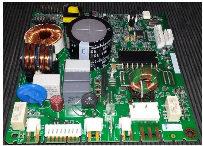
150W sensorless 3phase FOC driver of **BLDC** fan
