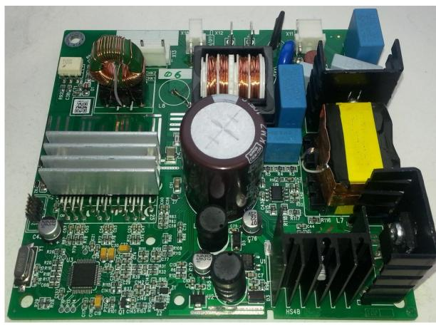
350W sensorless 3 phase FOC driver of **PMAC compressor**
